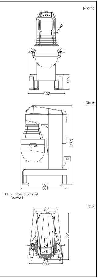
Supply voltage: 200-240 V/1N ph/50/60 Hz Electrical power, max: 2.2 kW **Total Watts:** 2.2 kW Capacity: ISO 9001; ISO 14001 kg/ Performance (up to): Cycle 40 litres **Capacity:** Key Information: External dimensions, 655 mm Width: **External dimensions,** Depth: 850 mm **External dimensions,** 1370 mm Height:
